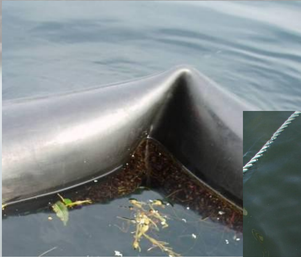
Permanent kinking of the HDPE pipe
