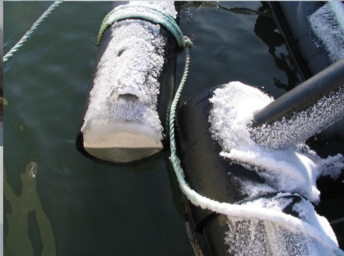
HDPE surface pipe broken
